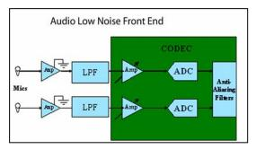
This typically starts with the front-end signaling, low noise audio design, and dynamic range scaling.
