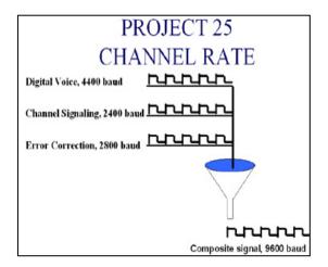
All of this processing puts continual pressure on reducing the data rate of the digitized audio. It is important to remember that one of the reasons to go digital is to improve the use of the transmitted spectrum. This only means one thing; limit the bandwidth of the transmission. An increase in the transmitted data rate will only increases the required bandwidth needed for transmission.
