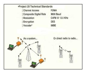
The Project 25 standard is based on being both digital and backward analog compatible with existing analog equipment. This standard provides for devices that can be used with both analog and digital systems.
