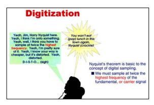
When we digitize the audio we want it, after converting it back to analog, to reflect the original sound. To do this we must sample the waveform often enough to capture all of the important changes and fluctuations of the audio signal. If we sample less often than is necessary, we will get a corrupted and incorrect representation of the audio signal.
