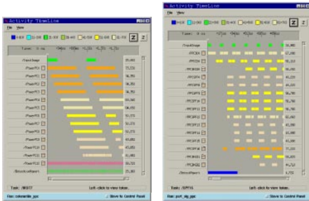
Figure 2: Utilization Versus Time for Partitioned Data (left) and Partitioned Algorithm Approaches Using the PowerPC
